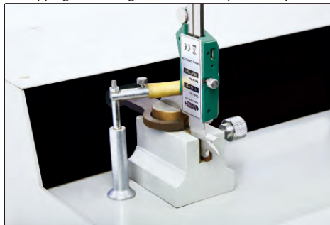
lapping measuring surfaces of caliper lower jaws
